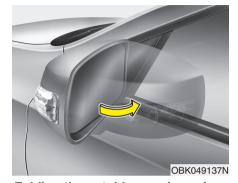
Folding the outside rearview mirror. To fold the outside rearview mirror, grasp the housing of the mirror and then fold it toward the rear of the vehicle.
