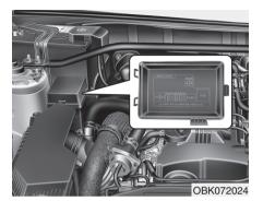
Engine compartment fuse panel
