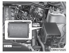
Engine compartment fuse panel
