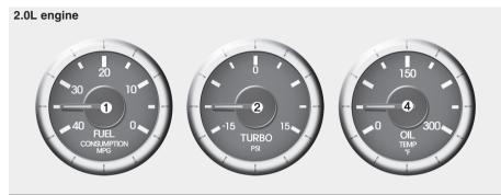
Multi gauge consists of a Instant fuel consumption gauge, turbo boost pressure gauge (for 2.0L engine), engine torque gauge (for 3.8L engine) and engine oil temperature gauge.
