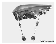
Turn signal light and side marker bulb replacement
