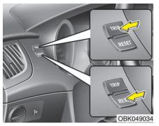
Tripmeter A or B can be selected by pressing the TRIP button for less than 1 second.
