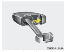
1. Insert a slim tool into the slot and gently pry open the cover.
